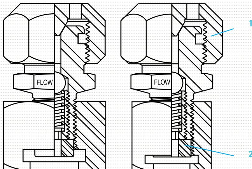
1 Steel Cap - Prevents leakage when unattended.
