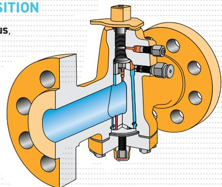
ALL OF THE SEALWELD® COMPOUNDS REFERRED TO MAY BE INJECTED USING SEALWELD® SEALANT INJECTION EQUIPMENT OR ANY OTHER TYPE OF HIGH-PRESSURE MANUAL OR PNEUMATIC INJECTION PUMP. **DO NOT USE LOW-PRESSURE AUTOMOTIVE PUMPS.**
