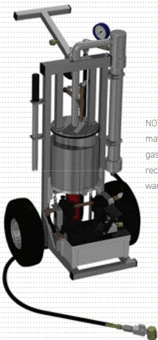
NOTE: The air/hydraulic motor may be powered by natural gas in an emergency, it is not recommended and may void warranty.
