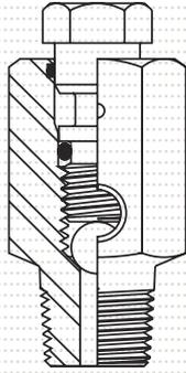
The standard body vent/ drain fitting does not allow for the removal of the stinger which is held in place with pins. This fitting is ideal for blowing-down ball valves or releasing pressure from the body of a gate valve during normal service.
