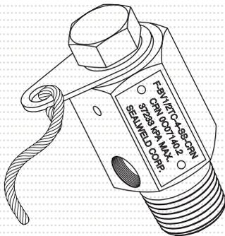
This design is similar to the TC3 in all respects with an added stainless steel ring and cable. It is designed to replace the existing carbon steel bleeder on hinged closures where plating failure has rendered the existing fitting inoperable.
