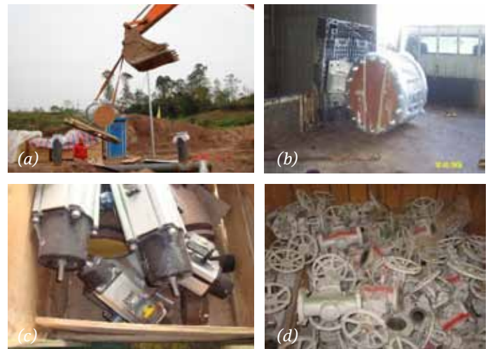
Figure 3: Examples of improper valve handling: (a) improper loading; (b) improper transportation; (c) improper packing; and (d) improper storage.
