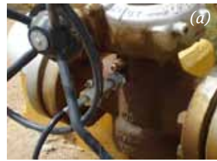
Figure 9: Examples of damage due to pipeline chemical cleaning: (a) chemicals attack the cover seal gasket, causing an external leak from a plug valve; and (b) chemical attack of a ball valve soft-seat insert.
