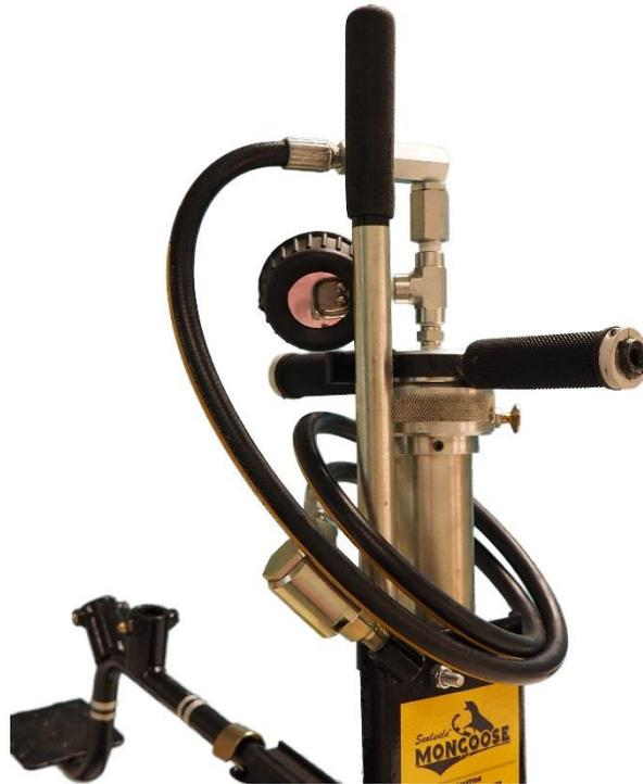
2. Keep the hose and L-swivel in place, insert the piston plunger into the receptacle loops found on vertical back plate.
