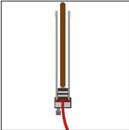
2. Remove the plastic wrapper from the stick of sealant. Use a screwdriver to make several grooves along the length of the stick of sealant. This will allow air to escape from behind the sealant as the stick is inserted into the barrel. When stick is fully inserted, the pump is loaded.
