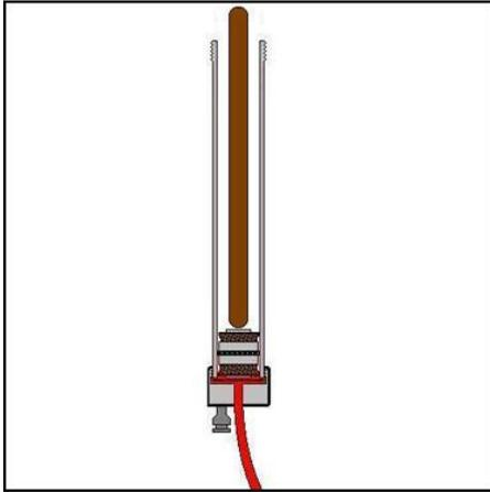
7. To "Break-In" the new cups and make loading easier, Repeat pushing the piston to the bottom then pumping it back up several times, Be careful not to pump the piston out of the barrel.
